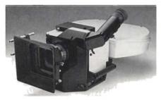
**Movement:** MSM Monoblock high-speed, triple register pins, claw engages four perfs. Shrinkage adjustment changes both stroke and entry position. Indexable loopsetting sprockets have independent locking keeper rollers. Vacuum backplate assures film plane accuracy, removes without tools for cleaning. Aperture and movement remove easily for cleaning and lubrication. Aperture size 1.485" wide x .992" high. Frame-rates from time-lapse to 72 fps forward, to 30 fps reverse.
